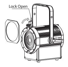
2. Slide the Barn Door in from the top, in front of the Gel Frame. The Barn Door will sit in the same slot as the Gel Frame
